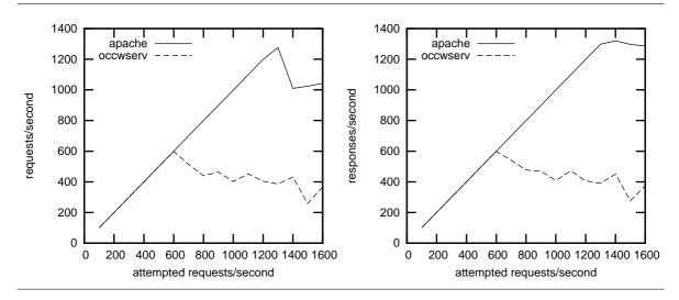
Figure 8: Request and response benchmark results (20,000 hits, 4 requests/connection, 8k static page)
