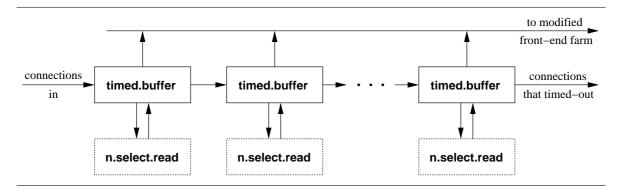
Figure 10: Example client request-reading process pipeline
