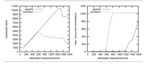
Figure 9: Network bandwidth and max. concurrent connections benchmark results (20,000 hits, 4 requests/connection, 8k static page)
