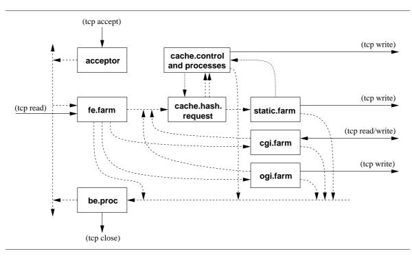
Figure 1: occam web-server main top-level processes
