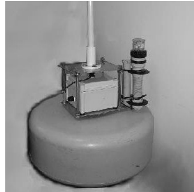
Fig. 6. Photograph of prototype buoy with mounted enclosure (white box) containing the radio and kOS modules. The antenna and navigation light are also shown. The submerged sensor module is not shown.
