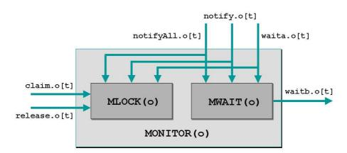
Figure 1: The Monitor Process (for Object  $\circ$ )
