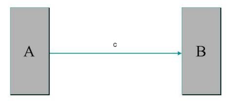
Figure 2: CSP channel communication
