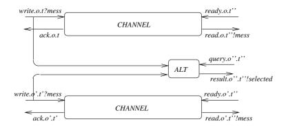
Figure 15: A 2-way ALTing Channel Version of Figure 10
