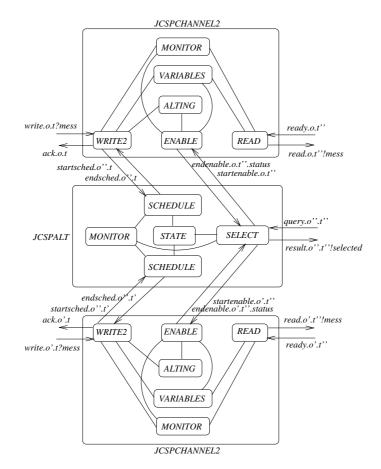
Figure 14: A 2-way ALTing Channel Version of Figure 11
