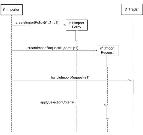
Fig. 1.4. Sequence diagram for ImportService use case
