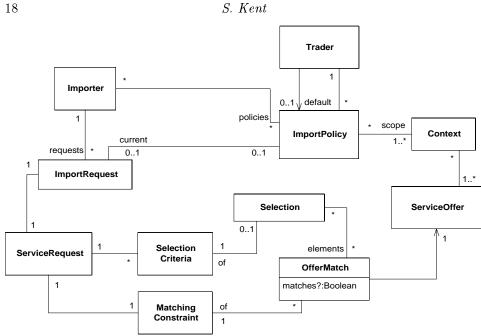
Fig. 1.5. Main class diagram for import service
