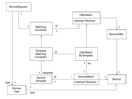
Fig. 1.6. Matching import requests to services: class diagram
