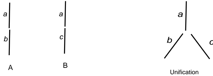
Fig. 4. Two simple behaviours defined as labelled transition systems and their unification according to extension
