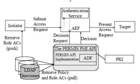
Figure 4: PERMIS API System Structure
