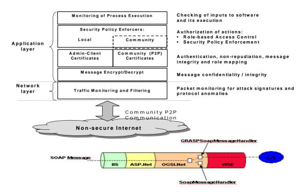
Figure 3. Overview of the GRASP distributed security enforcement architecture
