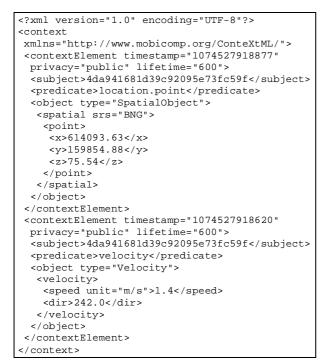
Figure 2. ConteXtML representation of MobiComp context elements for location and velocity.
