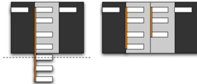
Figure 4.61: Visual-history : dealing with overflow. Left, An overflow of web pages, Right, the visual-history technique of dealing with overflow. Note that when using the visual-history technique, the light grey column extends itself, so that all nodes (representing links from a single website) are kept in the same cluster.
