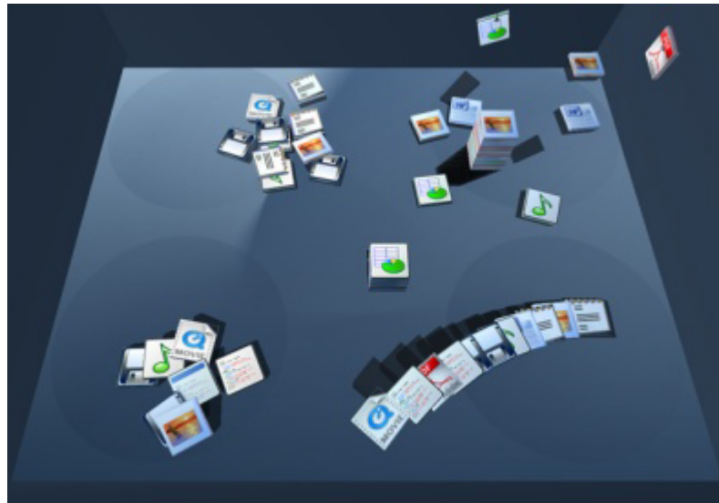
Figure 3.45: The BumpTop desktop metaphor (by Agarawala et al. [1]). This shows the three-dimensional desktop tool, BumpTop. The square tiles on the desktop represent files of different types. The physics of the desktop allow the files to be ‘picked up’ and ‘thrown’ around (or into corners) as if in real life. Files can also be ‘dropped’ on top of each other form ‘piles’ (like in real-life). This form of data management is easy to learn and use because of its inferences to real-life interactions.
