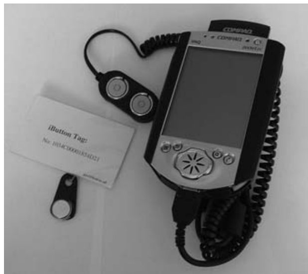
Figure 64. iPAQ equipped with an iButton reader.
