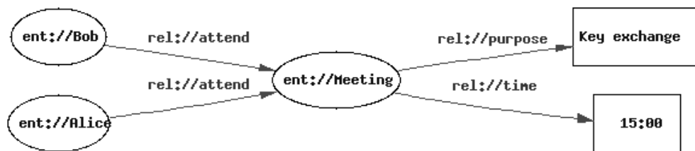
Figure 9. RDF Graph representing a simple context model
