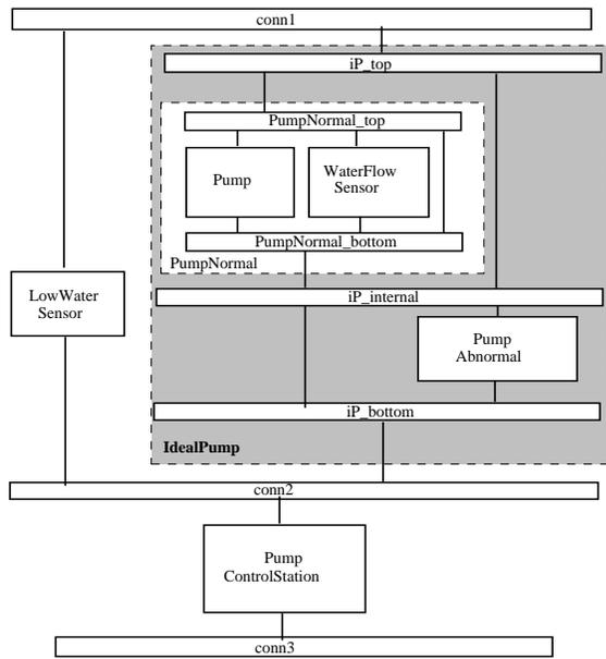
**Figure 5. C2 Configuration for Fault Tolerant PumpControlStation**
