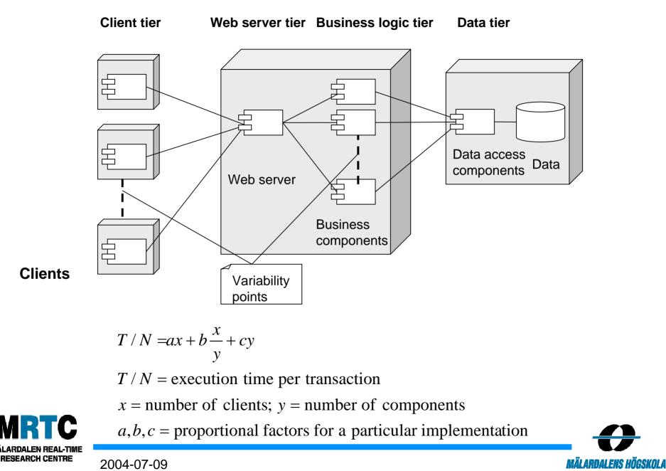
3. Definition: A derived property of an assembly is a property that depends on several different properties of the components.
