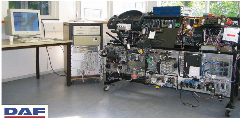
**Validator 2:** Commercial vehicle Hardware In the Loop testbench to prove EASIS dependability guidelines and development process
