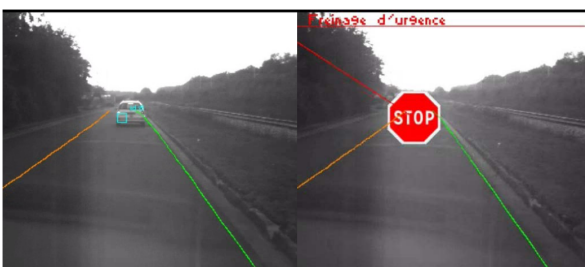
Figure 6. Emergency braking application screen capture
