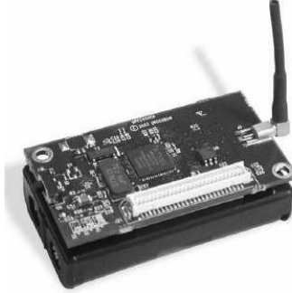
Fig. 7. MICAz mote used for localisation sensor
