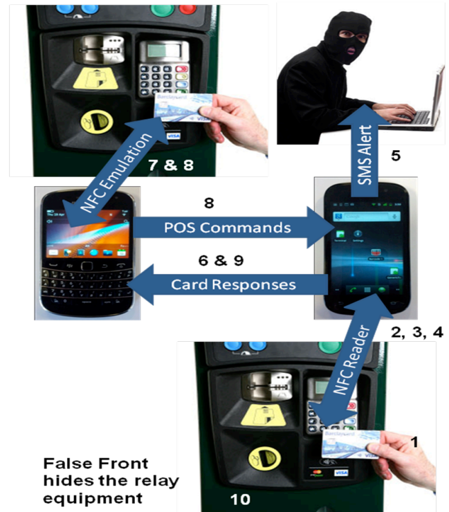
Figure 7. Parking Machine Attack
