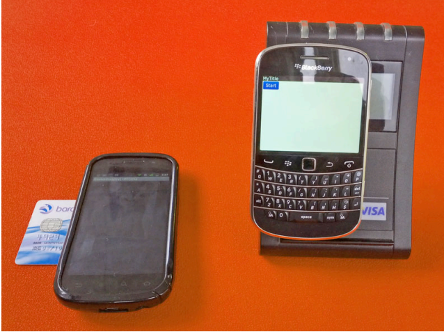
Figure 2. NFC Transaction Relay Using Mobile Phones
