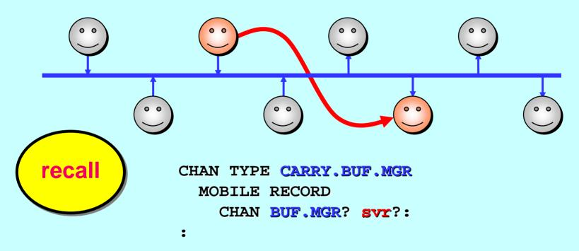
A *client* process makes both ends of a non-shared <code>buf.mgr</code> channel and *claims* the shared channel. When successful, it sends the *server-end* of its <code>buf.mgr</code> down the shared channel. This blocks until a *server* process *claims* its end of the shared channel and inputs that *server-end*.
