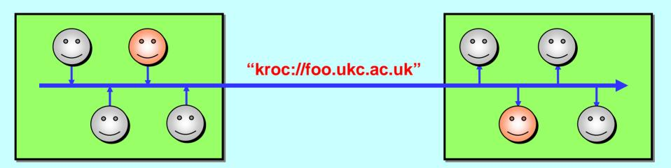
To set this up, the KRoC programmer (designer) only constructs the *named network channel structure* – the processes supporting the network are automatically forked and have no impact on system semantics.
