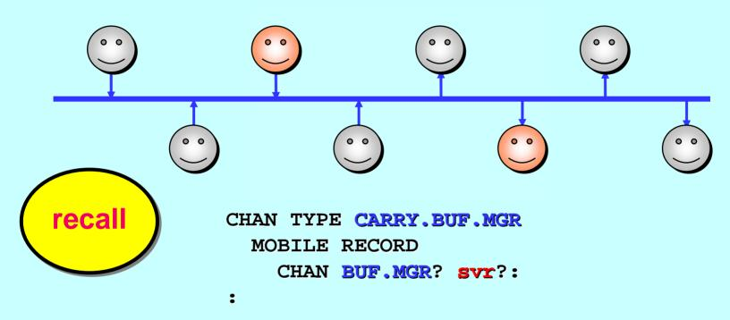
Once that *client* and *server* finish their business, the *server* should return the *server-end* of the <code>buf.mcr</code> channel back to the *client*, who may then reuse it to send to someone else. With a slightly modified definition of <code>buf.mcr</code>, its *server-end* may be sent down itself back to the *client*. ©
