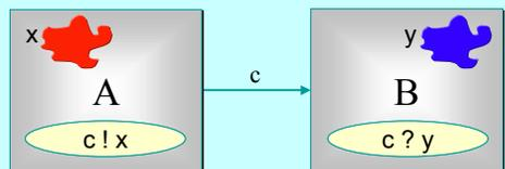
Only when both *A* and *B* are ready can the communication proceed over the channel *c* ...
