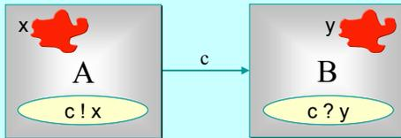
Only when both *A* and *B* are ready can the communication proceed over the channel *c* ... and it's happened!
