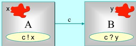
*Java/JCSP*: references to data (objects) are copied from the workspace of *A* into *B*. Subsequent work by *A* on its *x* variable and *B* on its *y* variable causes mutual interference (*race hazard*).
