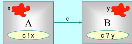
*Classical occam*: data are copied from the workspace of *A* into the workspace of *B*. Subsequent work by *A* on its *x* variable and *B* on its *y* variable causes no mutual interference.
