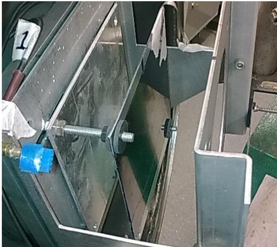
Figure 2.1.3: This image shows that the excess isolation tape from the mounting threads has been removed.
