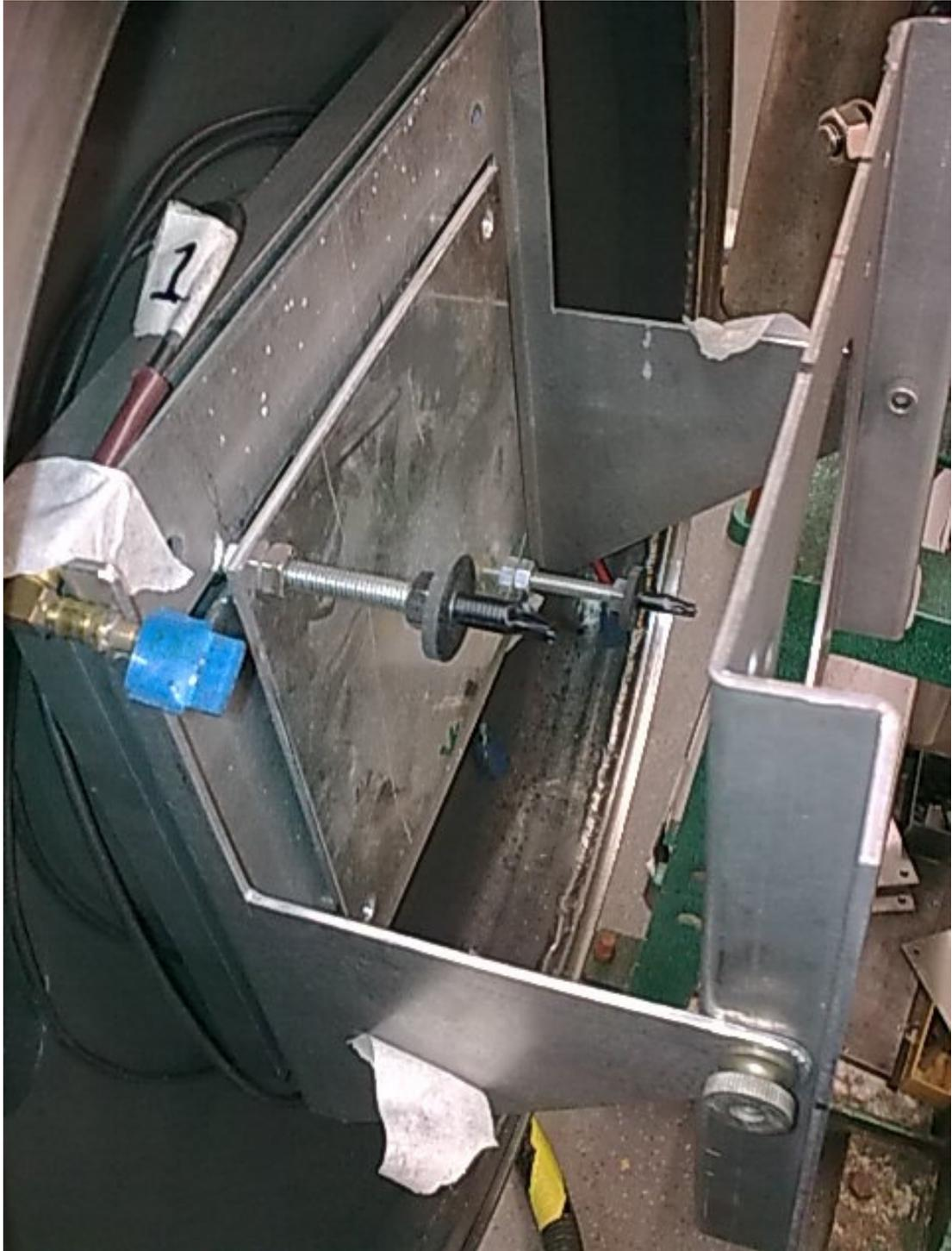
Figure 2.1.1: This is an image which shows the screws used to mount the rear plates. This image shows the rearmost plate already in position, and at the top of the screws there are one set of dampers in place, and the threads have been insulated. The mounting frame for the target plate can be seen on the right, in front of the mounting screws.
