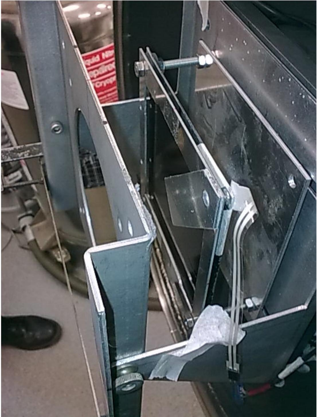
Figure 2.1.4: This image shows the shield frame mounted in front of the rear plate.
