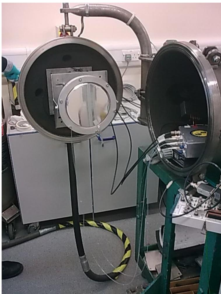
Figure 4.2: The FOMIS apparatus mounted within the door of the gun.
