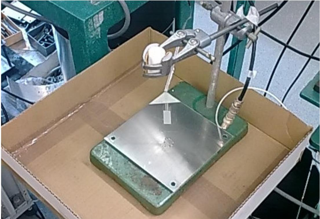
Figure 2.2.6: This is an image showing the use of a rear plate during bead drop testing, during the setting up of the apparatus. Rubber padding was positioned beneath the plate to isolate it.
