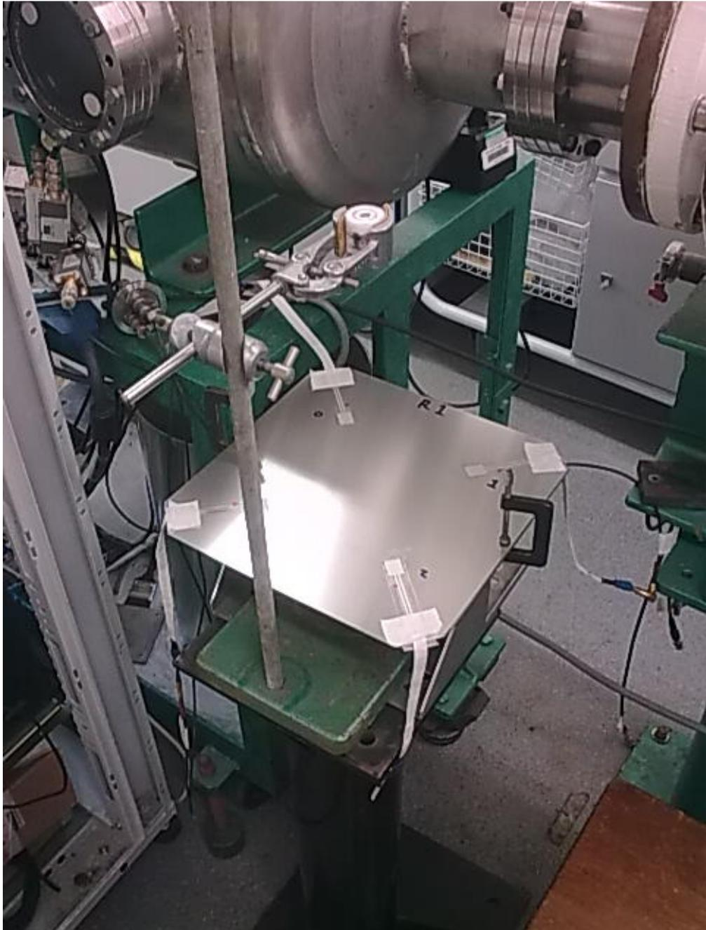
Figure 3.1: This is an image of an example of a plate undergoing bead drop testing. The free fall aperture has been positioned at the required height above the plate, and in such a position as to allow the ball bearings to impact the centre of the plate, at a point equidistant from all of the plate's PVDF sensors.
