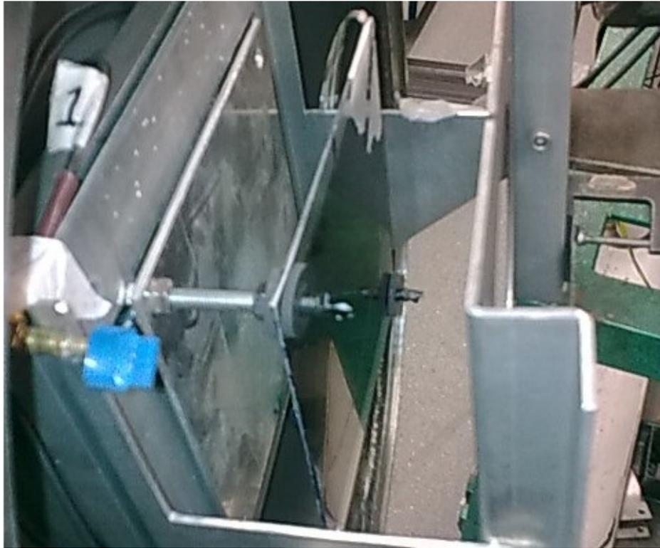
Figure 2.1.2: This image shows the rear plate mounted onto the screws. The second set of dampers have been added to the mounting, isolating the plate.
